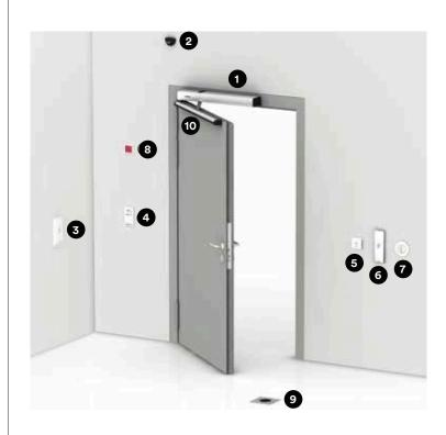
Automatic swing door systems from GEZE ease the access of a door every time when the manual opening is too hard or inconvenient. They are recommended in public as well as in private buildings, when convenience, accessibility, safety and hygiene are necessary or when energy has to be saved: in shopping centres, schools, office or industrial buildings, airports, clinics, vestibules or in private homes.
